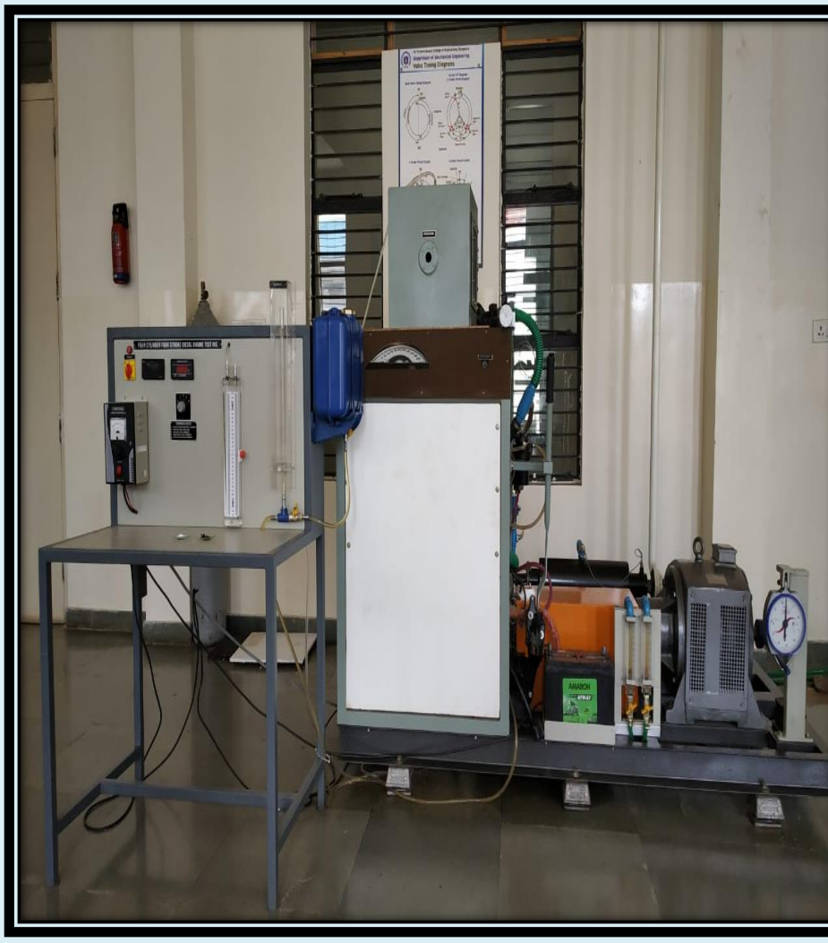
Multicylinder Diesel Engine Test Rig (Engine: Toyota Etios Model)
