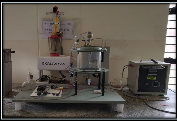
Biofuel Reactor (For Optimization of production parameters)
